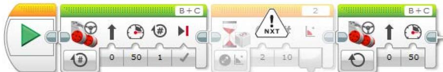
To use a Gyro Sensor as part of your Virtual Brick programs in the LEGO MINDSTORMS EV3 software, you can use the **RVW Gyro Sensor Block**. This block looks and acts exactly the same way as the default Gyro Sensor Block, but will work with the Virtual Brick and Robot Virtual Worlds:
